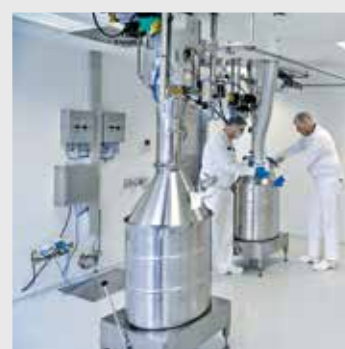
Powder collection in clean room, PHARMA-SD® type PSD-4.
