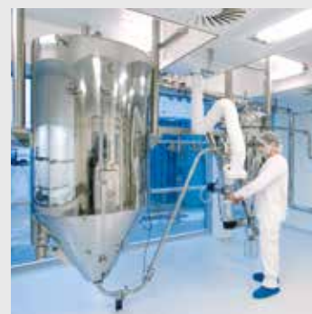
Custom-designed PHARMA-SD® type PSD-1 spray dryer in clean room.
