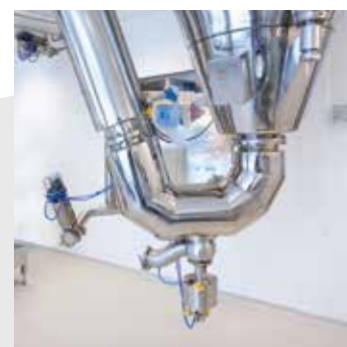
Cleaning-In-Place (CIP) requires a swing cone at the bottom of the drying chamber.
