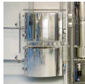
Filter housing for Bag-Out changing of HEPA filter element.
